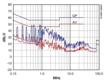
Figure 3. Conducted EMI scan to EN55022 B Limits. Measurements Made at 230 VAC With Output RTN Connected to Artificial Hand Representing Worst Case Conditions.
