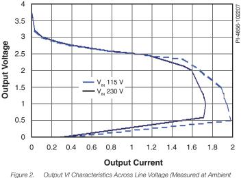
ure 2. Output VI Characteristics Across Line Voltage (Measured at Amb Temperature) .
