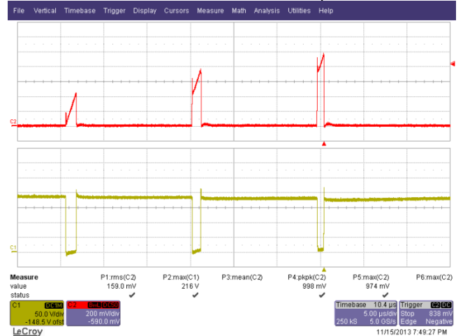
Figure 41 – 132 VAC, 60 Hz Output Short Condition. Upper: I_{DRAIN} , 500 mA / div. Lower: V_{DRAIN} , 100 V, 1 \mu s / div.
