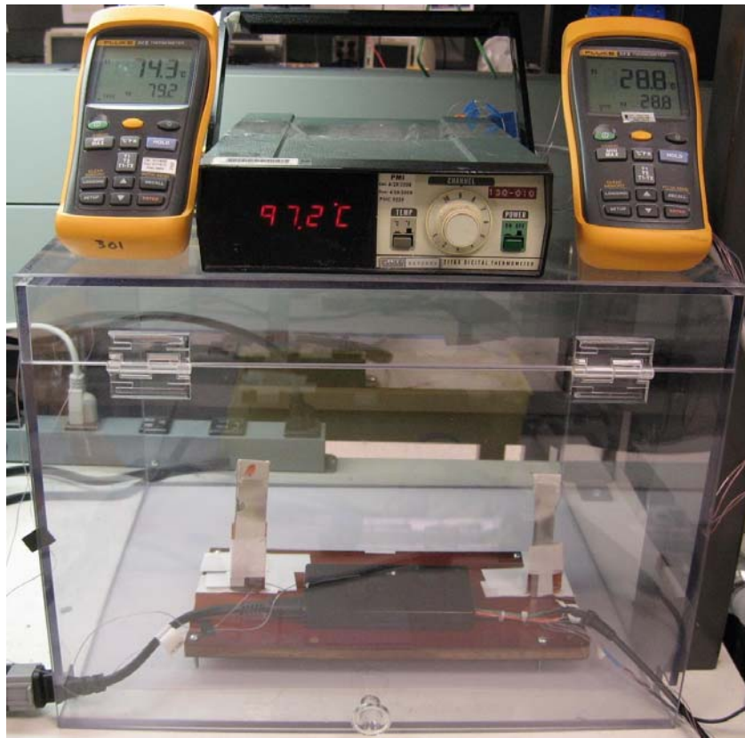
Figure 40 – Unit Placed on a Bakelite Board and Inside a Customer Specified Plastic-glass Chamber. Ambient Temperature: 28.8 °C; Case Temperature (Top): 74.3 °C; TOPSwitch Temperature: 97.2 °C.
