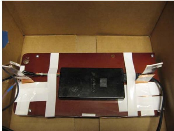
Figure 34 – Power Supply Adapter Inside Carton Box and on Top of Bakelite Board for Burn-In Test.
