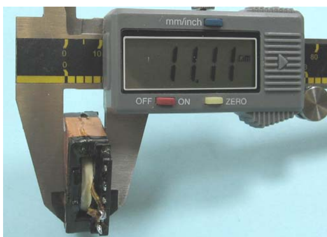
Figure 12 – Measured Height of the Complete Transformer.
