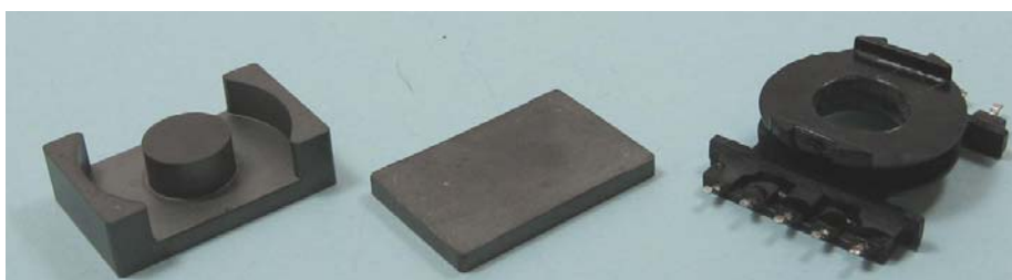
Figure 11 – Transformer Materials Showing EQ30, PLT30 Core, and Ultra-low Profile Wire-wound Bobbin.
