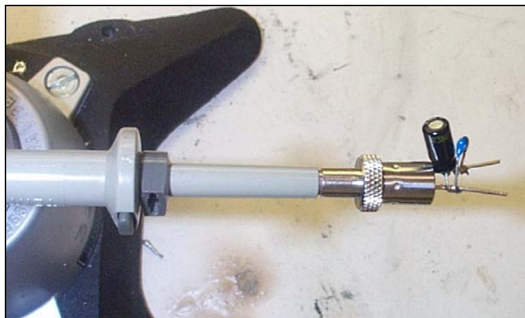
Figure 68 – Oscilloscope Probe with Probe Master 4987BA BNC Adapter. (Modified with wires for probe ground for ripple measurement, and two parallel decoupling capacitors added)
