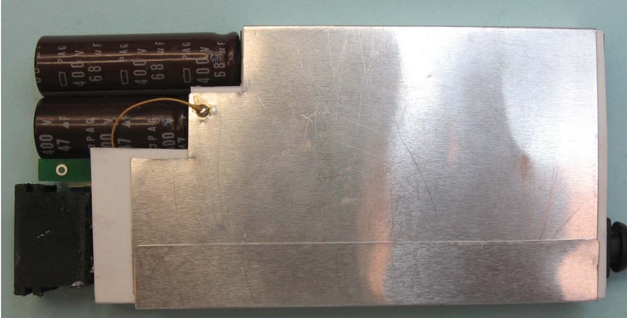
Figure 3 – Photograph of Assembled Unit with Heat Spreader in Place.
