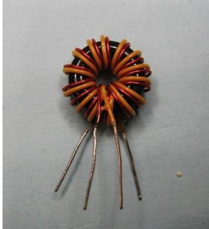
Figure 18 – 630 \mu H CMC Illustration Image.
