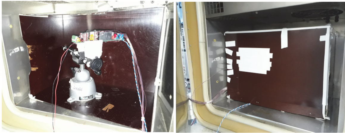
Figure 45 – Test Set-up Picture Thermal at 60 °C Ambient - Open Frame.
