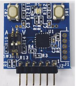
**Figure 1 –** Top view of InnoSwitch3-Pro Toggle Board.
