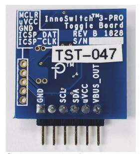
Figure 2 - Bottom view of InnoSwitch3-Pro Toggle Board.
