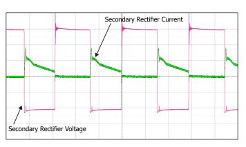
Figure 27. Secondary Rectifier Waveforms with Slow-Recovery Diode.
