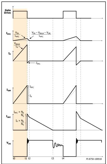
Figure 39. SVFS<sup>2</sup>PFC Timing Diagram, t0 to t1.
