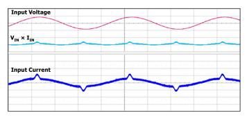
Figure 49. Input Current Waveform, SVFS<sup>2</sup>PFC + LYTSwitch-6 Flyback, 120 VAC
