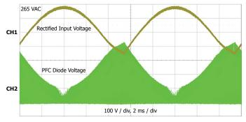
Figure 17. Voltage Stress across the PFC Diode.
