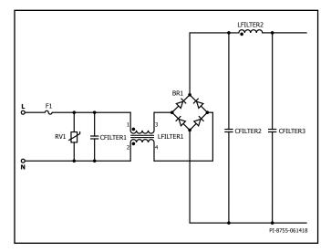
Figure 22. Input Filter Configuration in LYTSwitch-6 Designs.
