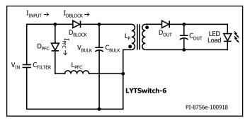
Figure 47. Input Current Flow, SVFS<sup>2</sup>PFC.
