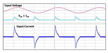
Figure 48. Input Current Waveform, Typical Non-PF Flyback, 120 VAC.
