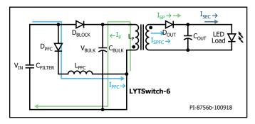
Figure 40. Current Flow from t1 to t2.
