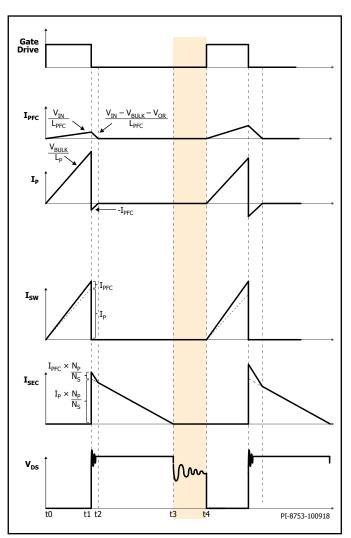
Figure 46. SVFS<sup>2</sup>PFC Timing Diagram, t3 to t4.
