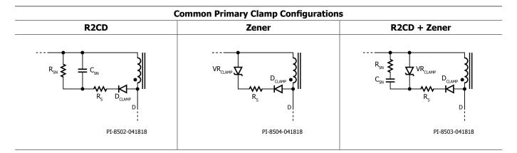
Figure 21. Recommended Primary Clamp Components.
