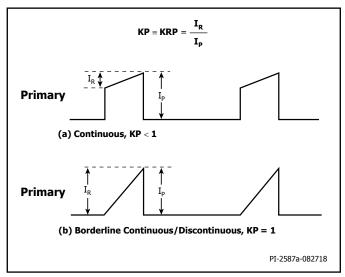
Figure 9. Continuous Conduction Mode Current Waveform, KP < 1.
