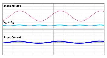
Figure 50. Input Current Waveform, SVFS<sup>2</sup>PFC + LYTSwitch-6 Flyback, 230 VAC.
