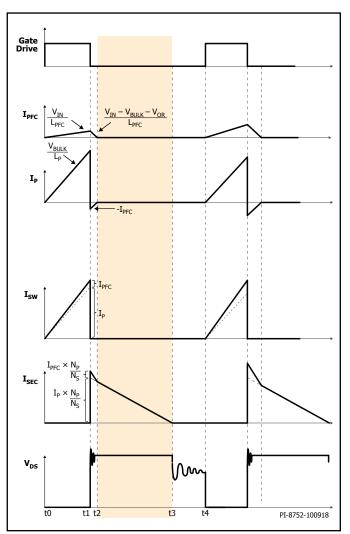
Figure 43. SVFS<sup>2</sup>PFC Timing Diagram, t2 to t3.
