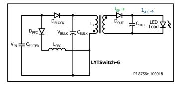
Figure 42. Current Flow from t2 to t3.
