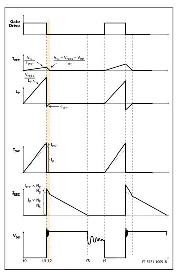
Figure 41. SVFS<sup>2</sup>PFC Timing Diagram, t1 to t2.
