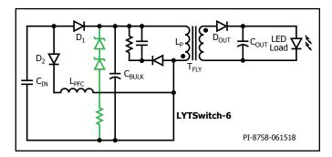
Figure 25. Zener Clamp Connected Across Bulk Capacitor.
