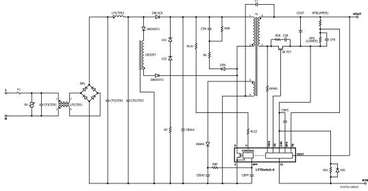
Figure 1. Typical Application Schematic for  $V_{o} < 24$  V.
