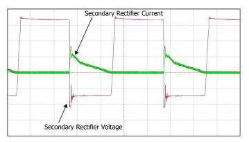
Figure 28. Secondary Rectifier Waveforms with Ultrafast Diode.
