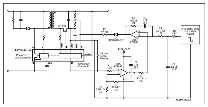
Figure 32. PWM Circuit.
