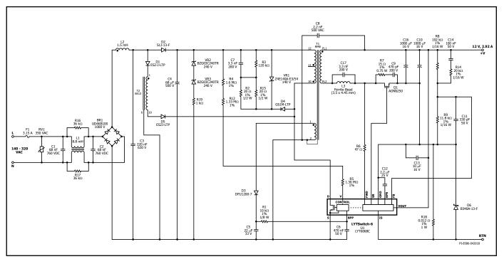
Figure 34. Schematic of DER-637, 35 W, 12 V, 2.92 A, 140 VAC – 320 VAC using LYSwitch-6 LYT6068C with Synchronous Rectification.
