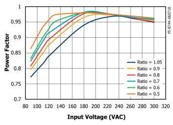
Figure 12. Power Factor vs. RATIO\_LBST\_LFB.
