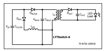
Figure 36. Simplified SVFS<sup>2</sup>PFC Schematic.
