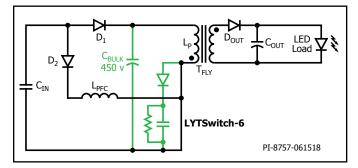
Figure 24. RCD Clamp Connected from Drain to Source.
