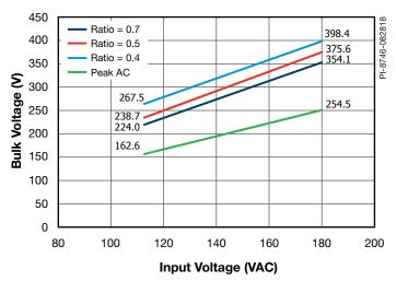
Figure 23. No-Load Bulk Voltage vs LPFC/NOM Ratio.
