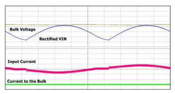
Figure 51. Bulk Voltage Waveform, SVFS<sup>2</sup>PFC + LYTSwitch-6 Flyback, 230 VAC.
