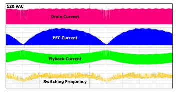
Figure 45. Current Waveforms, 1 Line Cycle.
