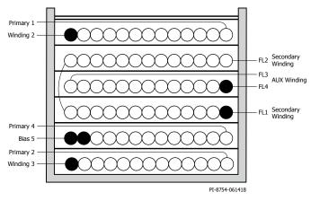
Figure 26. Sandwiched Secondary Auxiliary Winding Transformer Construction.
