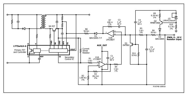
Figure 33. 3-in-1 Dimming Circuit.
