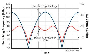
Figure 8. LYTSwitch-6 + SVFS<sup>2</sup>PFC Switching Profile (Simulated).
