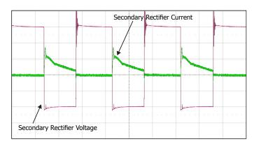
Figure 29. Secondary Rectifier Waveforms with Ultrafast Diode and Sandwiched Auxiliary Windings.
