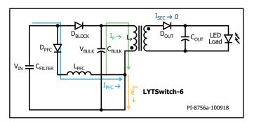
Figure 38. Current Flow from t0 to t1.
